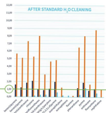
STUDY 2: TOXICOLOGICAL PROFILE OF FIRE GEAR AFTER STANDARD CLEANING WITH WATER AND DETERGENTS After cleaning the gear according to a standard cleaning process with water and detergents (18 different programs were tested), there was still an amount left in the gear of 92,28mg/kg, what is 9 x higher than the standard. The contaminants after standard decontamination, the main contamination is still found in the membrane (~90%).
